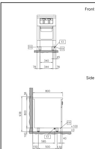
EI = Electrical inlet (power) EQ = Equipotential screw
